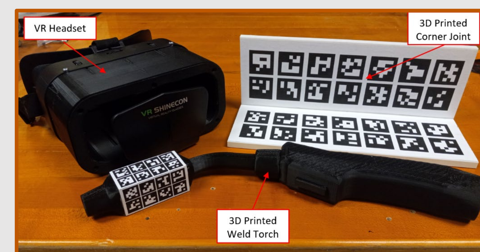
Figure 1: 3D Printed VR headset with markers for simulation
